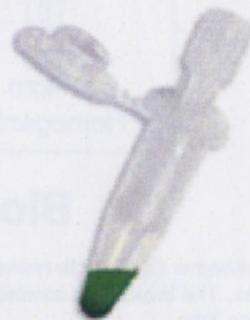
The BioMasher is an essential tool for any researcher working with protein and nucleic acid extraction. Its proprietary design consists of a homogenizer for grinding your sample, a column for straining, and a collection tube to contain the final homogenate. This system can be used on a wide variety of tissues, and is an ideal preparatory step for many downstream applications.
